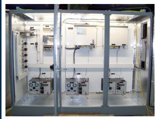
This system is an example of a multi-point continuous CO measurement. PRB coal is a much more volatile solid fuel and therefore the use of a stream switching system should be avoided.
